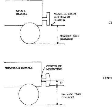
MANUFACTURER'S STOCK ORIGINAL DROP BUMPER MOUNTING 3" CENTER OF ALTERNATE MOUNTING MEASURE FROM Measure this BOTTOM OF BUMPER distance NONSTOCK DROP BUMPER MANUFACTURER'S ORIGINAL MOUNTING 3″ CENTER OF ALTERNATE MOUNTING 5" Measure this distance
